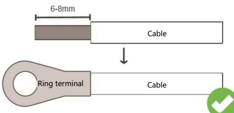
The cable size is for reference only. If the distance between the PV array and the inverter or between the inverter and the battery is long, using thicker cables will reduce voltage drop and improve system performance.
